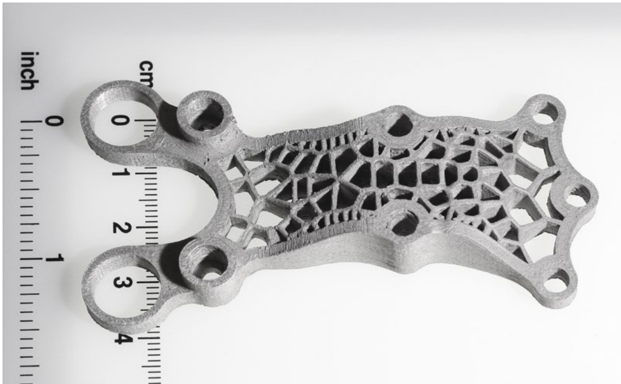
Fig. 3 Supporting element manufactured by MEX in 17-4 PH stainless steel after debinding and sintering
